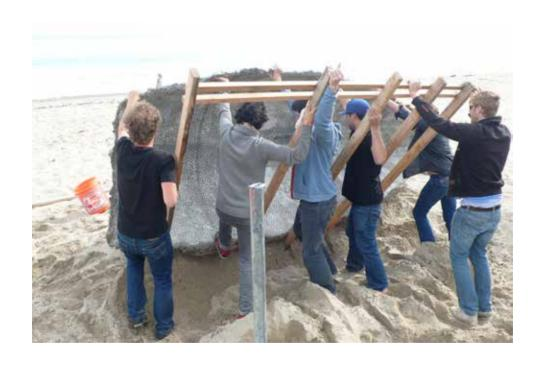
The hull is turned onto a mound of sand.
