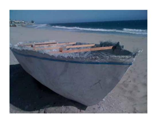
The inside and top edge are now complete and the hull is braced for transport.
