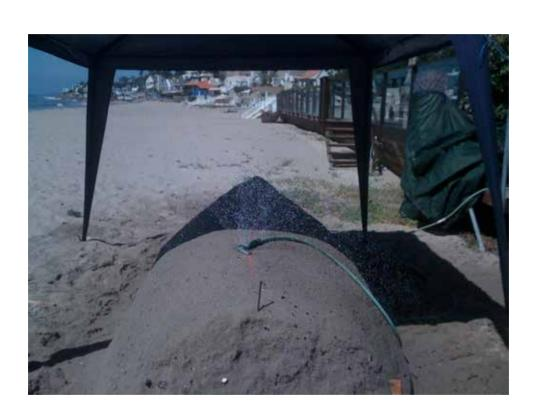
Only wet sand remains wet. Any dry sand within the pile will remain dry as the water follows the path of the already wet sand.
